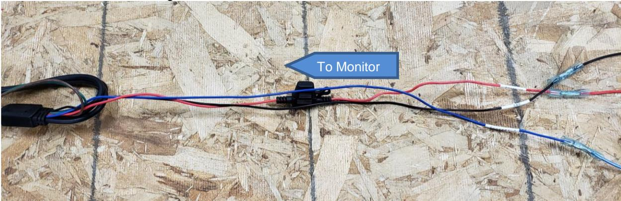
2. Begin to insert Field Fix by cutting into wires and connecting to attached Butt-connectors, as show below:
