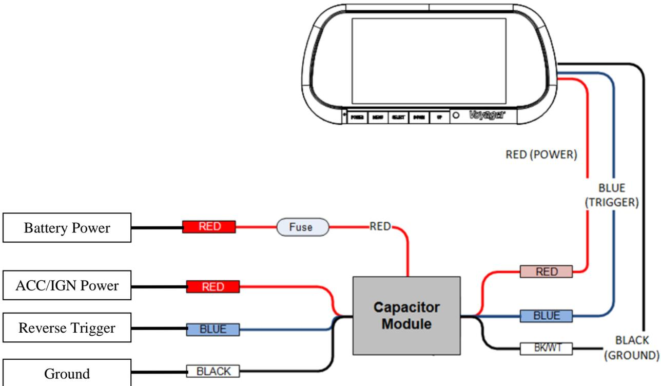
**\*It should be noted that the Blue Trigger Wire is a 'Pass Through Wire' and is not required for the Field Fix Component. This Pass Through Wire allows for easier insertion of the wiring harness depending on vehicle wiring, otherwise it doesn't need to be used and the present Trigger Wire can be left alone.**
