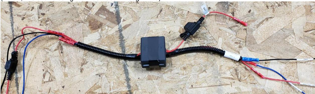
3. The Battery Wire then needs to be attached to a Battery/Constant Battery source. This could be achieved by attaching a ring terminal to a Battery Terminal at the Battery location or splicing into a Battery Wire with a Butt-connector.
